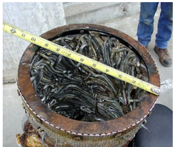
FIGURE 18. Larvae/juvenile lamprey entrapped in turbine water cooling screen from mainstem dam.
