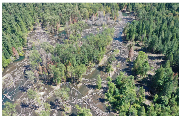
Figure 3. Pre-project conditions (left) as a single-thread transport channel and one year post-project conditions (right) with maximum valley connectivity and complexity.
