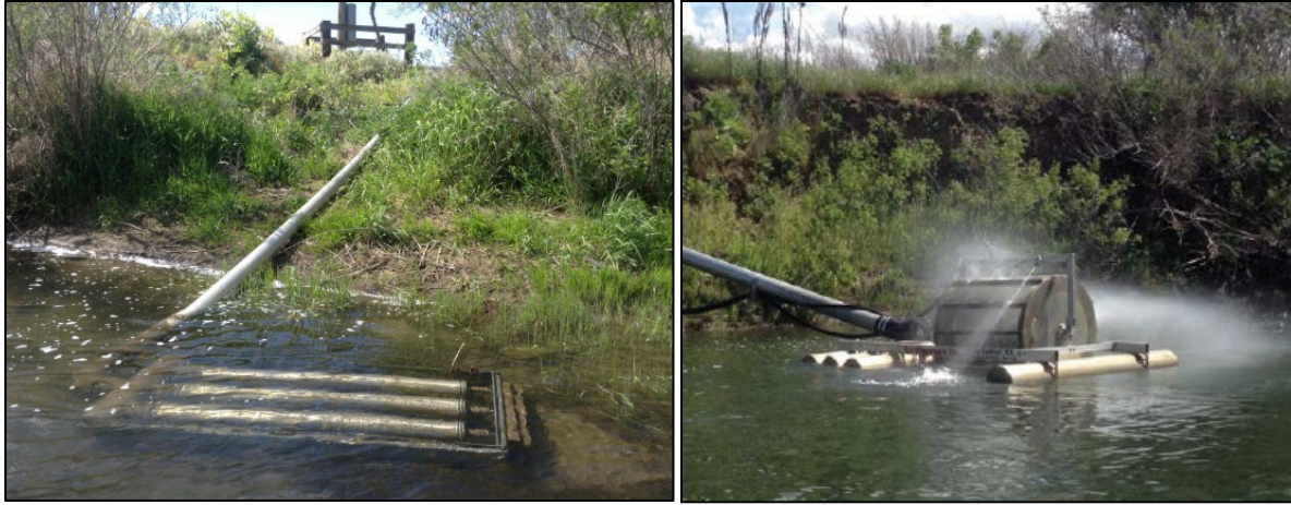
Figure A-7. Two examples of pump screens. Pump Rite manifold (left) and a Riverscreen (right).
