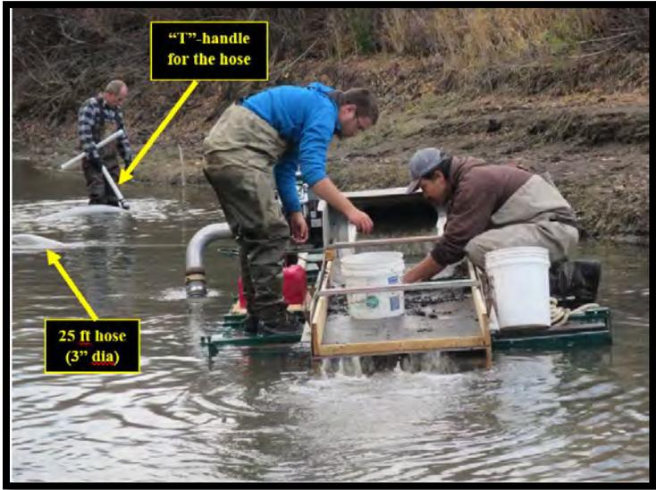
**Figure 4.15.** The sluice box in operation. “T”-handle used to maneuver the 4-inch suction hose for fine sediment and larval lampreys. With the heavy pump on side side, the sluice box tended to sink down on that side when a crew personnel also stood on that side.
