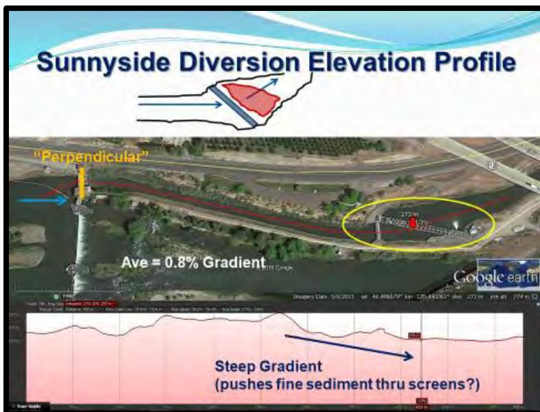
**Figure 6.26.** Sunnyside Diversion canal configuration between headgate and fish screens. The channel is straighter compared to Wapato Diversion and the average gradient is steeper (0.8%) with the steepest section right in front of the fish screens.
