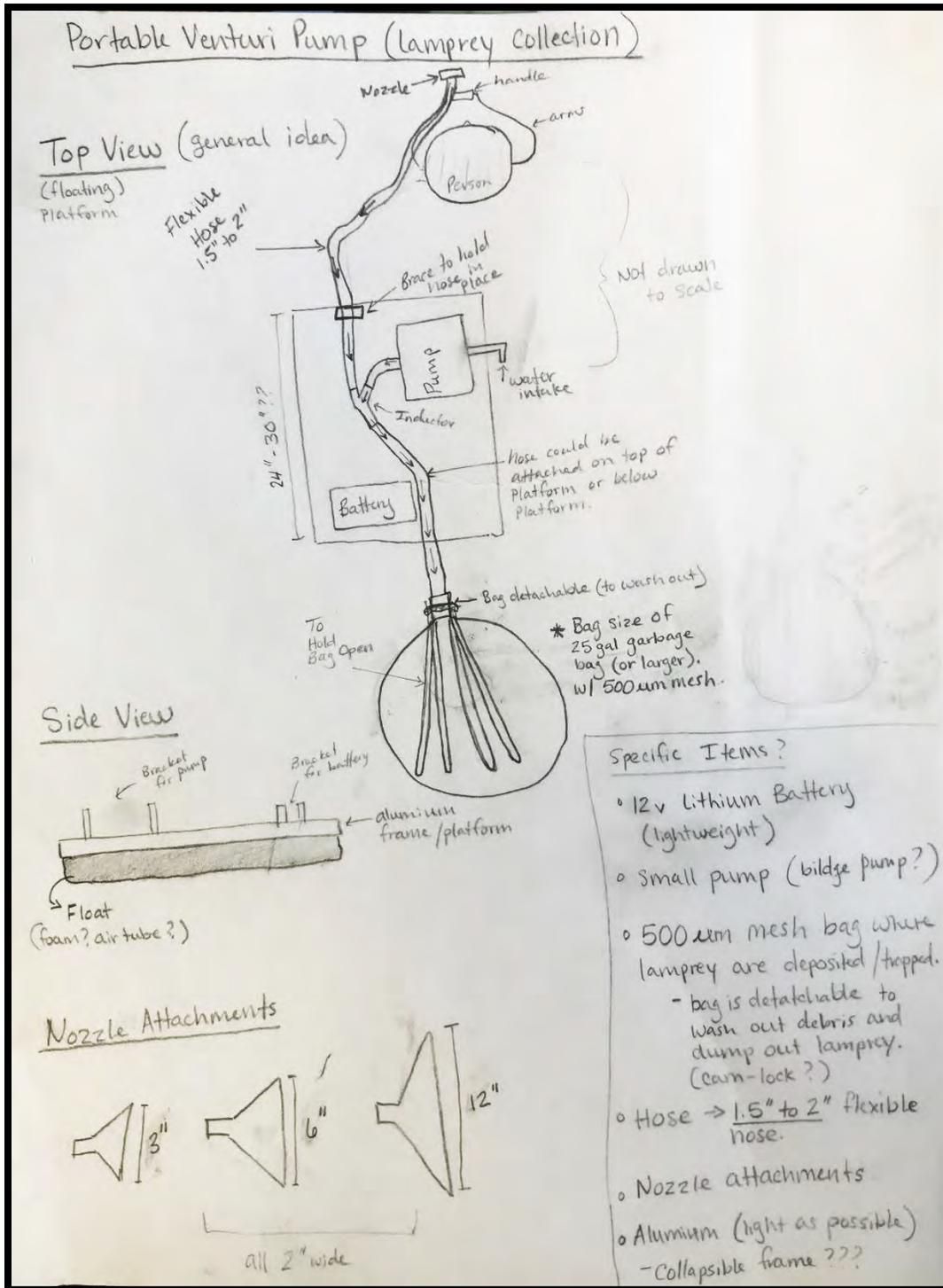
**Figure 4.21.** Another conceptual design for a portable lamprey sifter that uses a small scale venturi pump in combination with an electrofisher. After the electrofishing forces larval lampreys to emerge, the lamprey sifter will siphon lampreys into an expandable mesh bag (500-750 micron), which can be sifted in water if any fine sediment is also collected. A few nozzle attachments will be available to allow for the most efficient lamprey collection based on canal water height.
