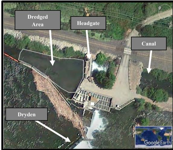
**Figure 4.10.** Area dredged in the forebay of Dryden Diversion on the Wenatchee River (RKM 27.8, Dryden, WA).
