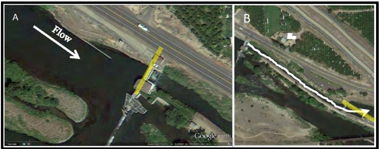
**Figure 6.24.** A) Overview of the inlet to Sunnyside Diversion displaying the orientation of the headgate (yellow) relative to the direction of the main channel flow. B) Overview of the flow direction between the headgate and the fish screens.
