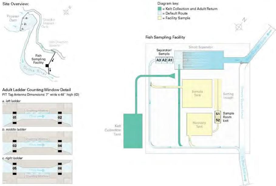
**Figure 3.4.** The PIT arrays located at Chandler Juvenile Fish Monitoring Facility (CJFMF).
