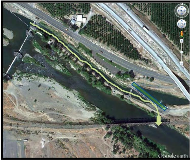
**Figure 7.5.** A conceptual model of using an irrigation diversion upstream of the fish screens as a “perennial side channel” with water returning through the bypass channel (yellow line tracing the flow direction with the arrow pointing to the bypass return flow). Water would have to be blocked at or near the fish screens (yellow polygon) so that no water can permeate downstream of the screens into the canal.
