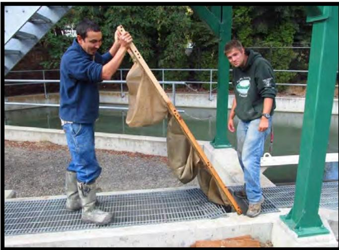
**Figure 3.24.** Inserting a custom made net for the trap efficiency test in the bypass channel.
