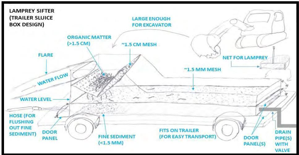
**Figure 4.17.** A lamprey sifter that will fit on a trailer. It has a sluice box with two built in mesh sizes: a coarse mesh (~1.5 cm) that will hold coarse organic material while larval/juvenile lampreys pass through and a fine mesh (~1.5 mm) that will hold the majority of larval/juvenile lampreys while fine sediment will pass through.
