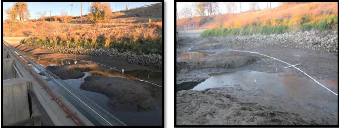
**Figure 5.8.** Overview of the sprinkler system operation downstream of the fish screens at Sunnyside Diversion immediately after dewatering of the key larval lamprey habitat occurred. Part of the sprinkler system was able to cover the high density isolated pools.
