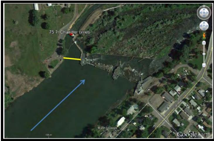
**Figure 6.20.** Chandler (Prosser) Diversion on the Yakima River (inlet angle = 45 degrees, canal width = 11 m). The blue arrow displays the thalweg flow direction and the yellow line displays the general orientation/angle of the headgate structure.
