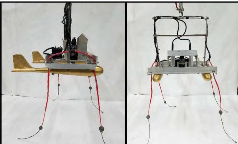
**Figure 3.11.** Portable deepwater shocking platform (side and front view).
