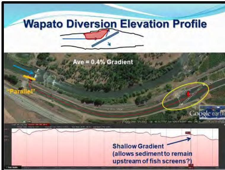
**Figure 6.25.** Wapato Diversion canal configuration between headgate and fish screens. The channel is not as straight as Sunnyside Diversion (curves to the left) and the average gradient is shallower (0.4%) with the shallowest gradient found in front of the screens.
