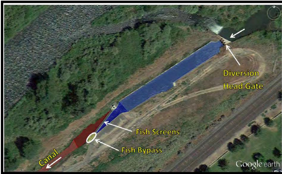
**Figure 6.4.** Overview of Selah-Moxee Diversion (Yakima River) displaying the four key areas: Above screens canal (light blue), above screens (dark blue), below screens (dark red), below screens canal (light red) (see Table 1 for more information). Key structures in the photo are also labeled.
