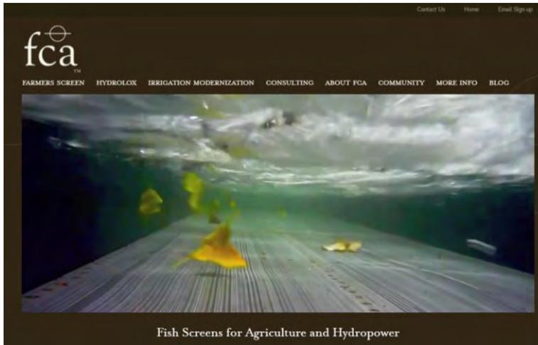
**Figure 7.1.** Underwater view of Farmers Screen, which is a horizontal, passive fish screen design that uses hydraulics to manage debris and protect fish. It has no moving parts and does not require power to operate. The Farmers Screen is a patented technology licensed solely to FCA (<https://farmerscreen.org/>).
