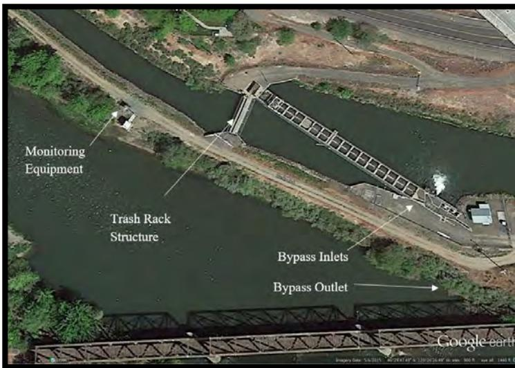
**Figure 1.1.** Illustration of Sunnyside Diversion channel and diversion infrastructure.
