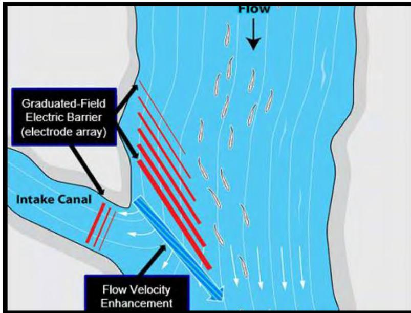
**Figure 7.3.** A conceptual design for combining the Graduated-Field Electric Barrier system and the Flow Velocity Enhancement system to exclude migrating fish from water intake structure and guide them safely downstream.
