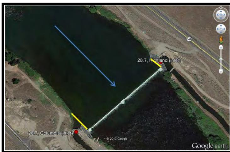
**Figure 6.19.** Columbia Diversion (left) (inlet angle = 90 degrees, canal width = 8 m) and Richland Diversion (right) (inlet angle = 90 degrees, canal width = 9 m) on the Yakima River. The blue arrow displays the thalweg flow direction and the yellow lines display the general orientation/angle of the headgate structures.
