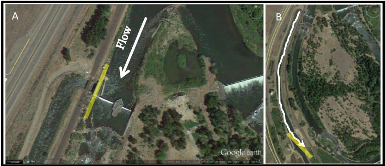
**Figure 6.23.** A) Overview of the inlet to Sunnyside Diversion displaying the orientation of the headgate (yellow) relative to the direction of the main channel flow. B) Overview of the flow direction between the headgate and the fish screens.
