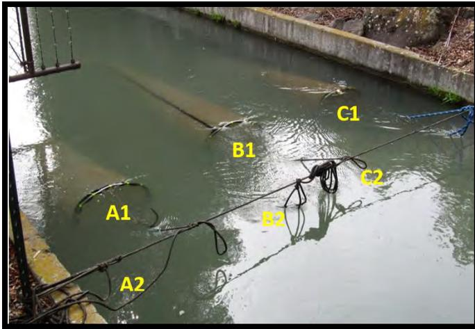
**Figure 3.25.** Three 0.5 m plankton nets placed in the upper water column inside the canal outlet channel to test the trap efficiency. “A1”, “B1”, and “C1” refer to the position of the net in the upper water column. When nets were placed on the bottom of the water, they were referred to as “A2”, “B2”, “C2.”
