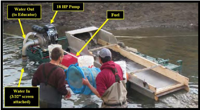
**Figure 4.14.** Side angle view of the sluice box system with labels for pump and associated parts.
