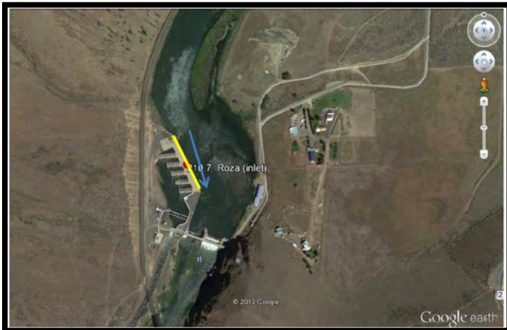
**Figure 6.21.** Roza Diversion on the Yakima River (inlet angle = 80 degrees, canal width = 6 m). The blue arrow displays the thalweg flow direction and the yellow line displays the general orientation/angle of the headgate structure.
