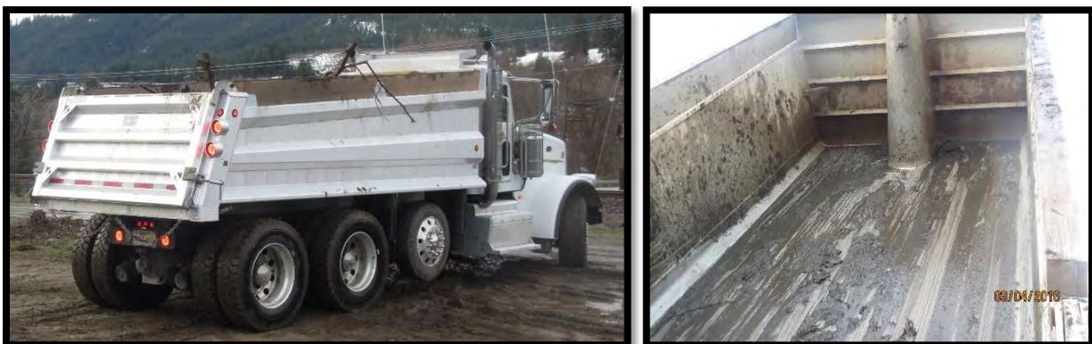
**Figure 4.12.** Custom-made waterproof dump truck owned by Wilsonville Concrete Products (Wilsonville, OR). Overview (left photo) and the inside (right photo).
