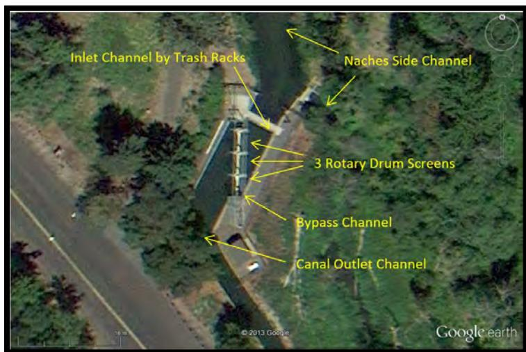
**Figure 3.21.** An aerial map of Congdon Diversion with labels for key components.
