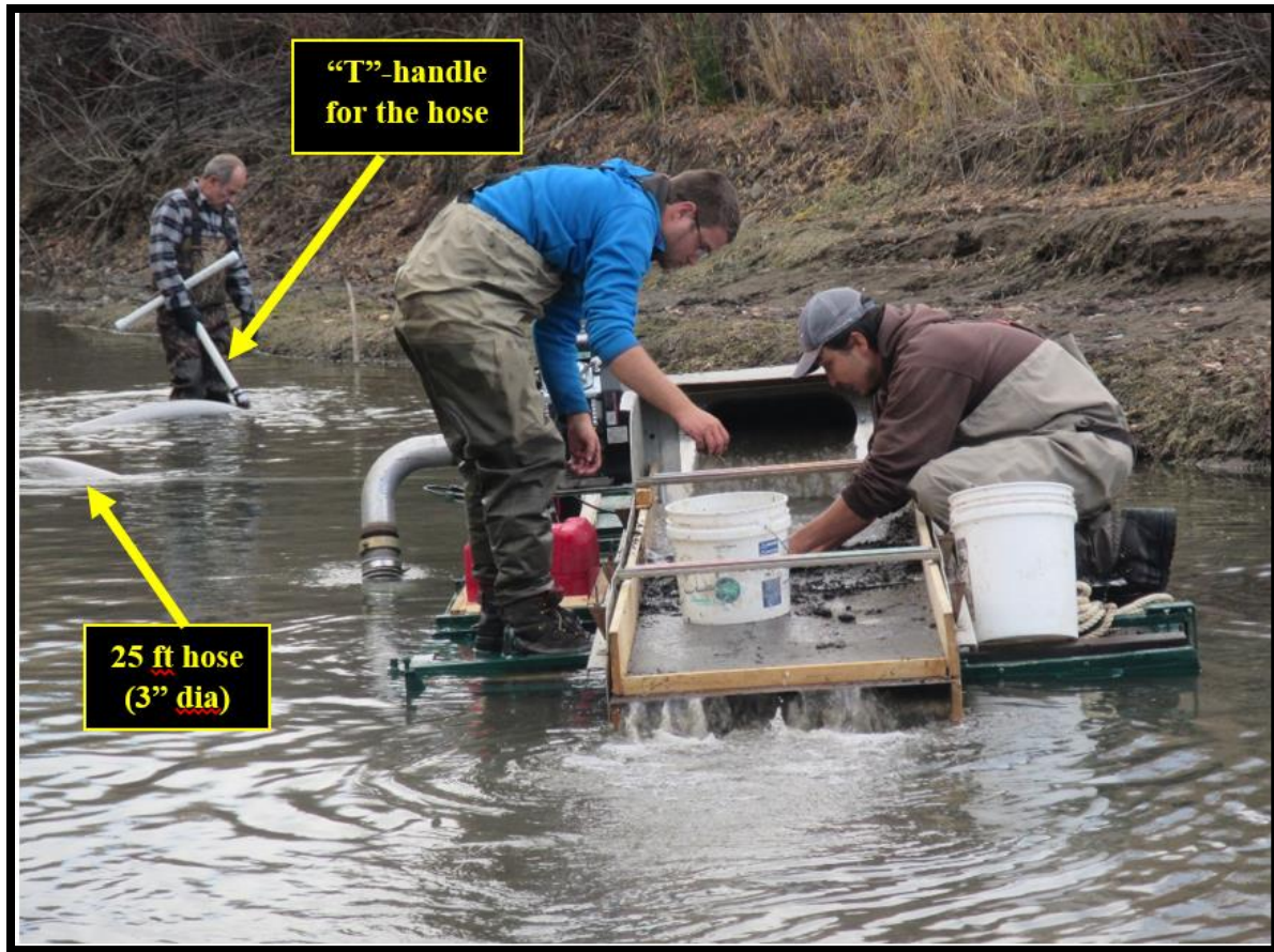
Figure A-5. The sluice box in operation. “T”-handle was used to maneuver the suction hose. The weight of the pump on one side created the potential for imbalance.
