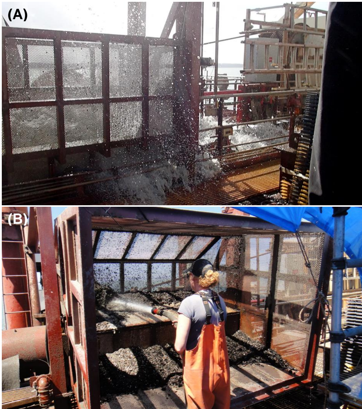
Figure A-3. Basket used to collect dredged material on the hopper dredge Essayons . (A) shows the basket being filled during dredging; (B) shows dredged material being washed from the basket while looking for entrained organisms.
