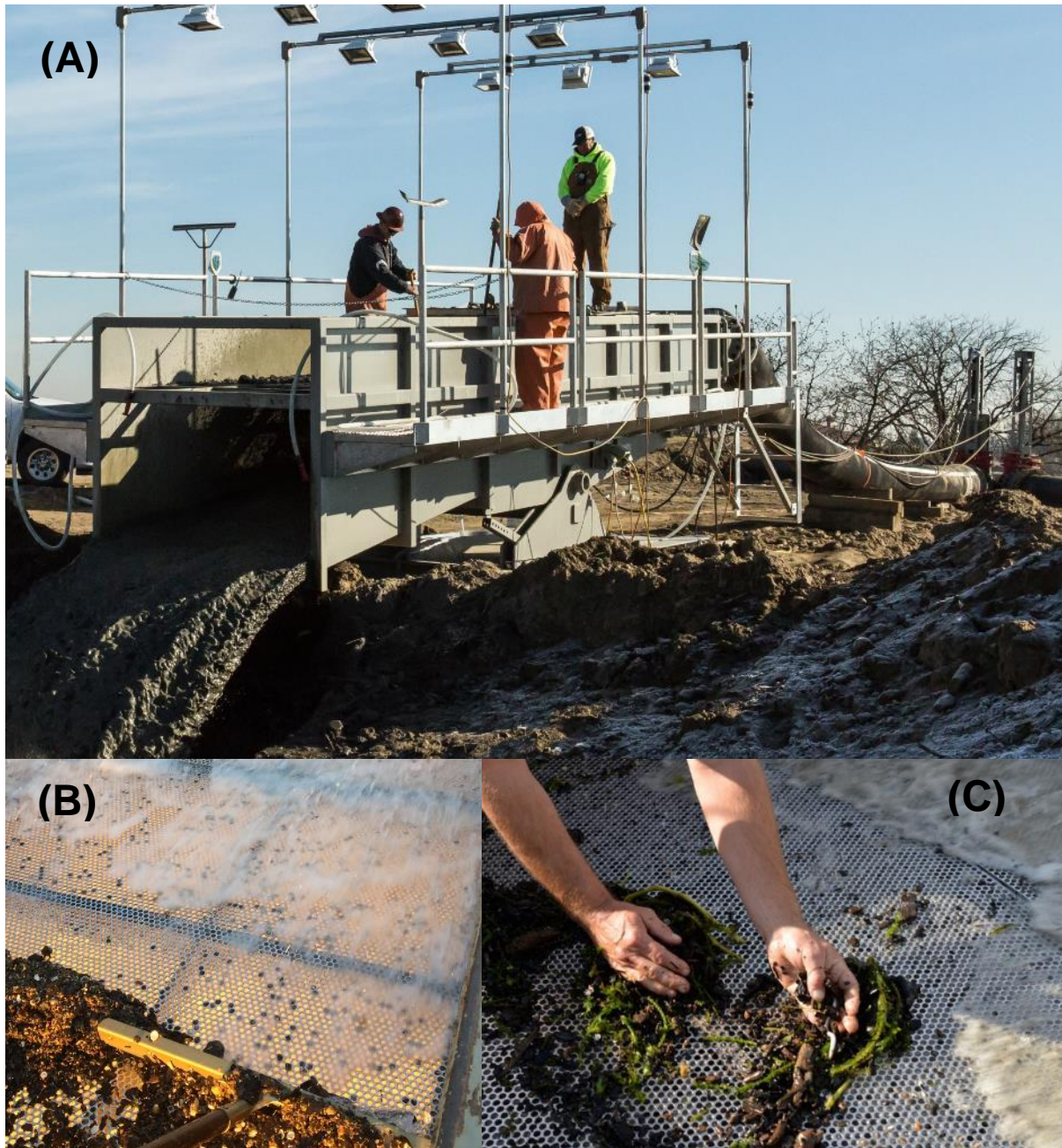
Figure A-2. A screening device used to monitor cutterhead dredge material. (A) shows the screen connected to the dredge discharge pipe with material flowing through; (B) shows water and dredged material flowing over the screen; (C) shows examination of dredged material for fish and other organisms.
