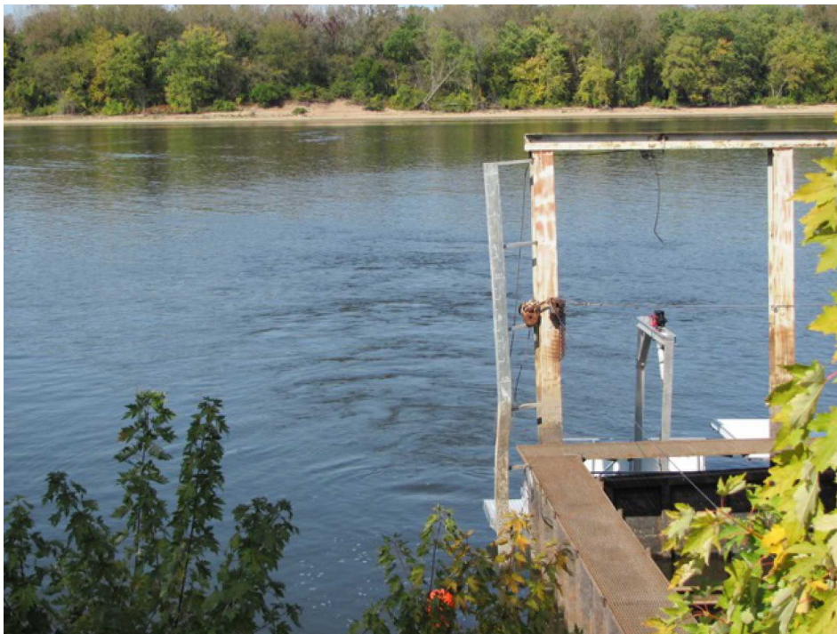
Figure 2. Surface view of a turbulent velocity plume in the upper Mississippi River from a FVES unit placed under the orange float at bottom of photo (low river flow from right to left).
