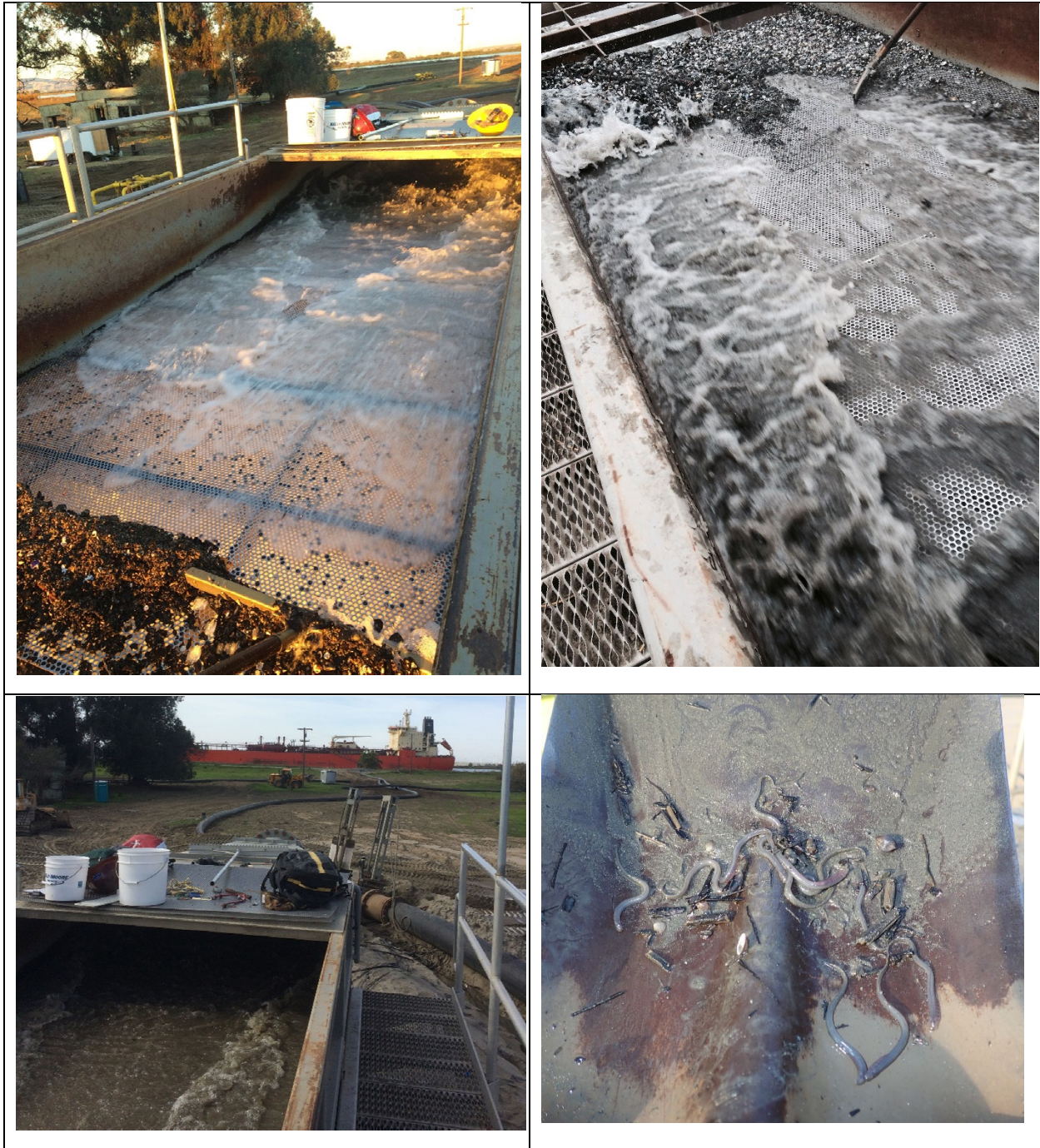
Figure 4. Overview of lamprey sifter developed by Jordan Gold (Mari-Gold Environmental Consulting, Inc.) and used in California.
